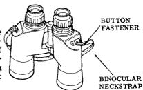
Replacing Binocular Case Shoulder Strap (NSN 1240-00-253-5892)
