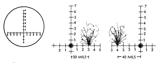
Fire corrections can be made by viewing the impact area and determining angular corrections by use of the left or right horizontal reticle scale.
